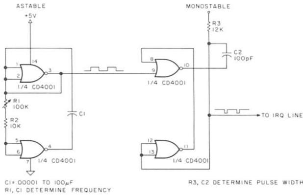
Fig. 1. Interrupt-oscillator circuit.
