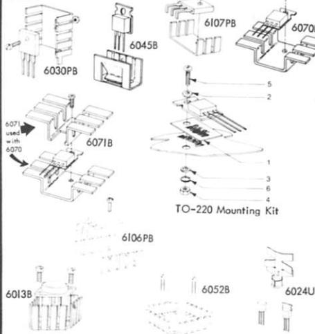
Economical 1 piece heat sinks for plastic power parts in TO-220 and Motorola cases 77, 90, 199, and TO-126. All are black anodized aluminum. "B" series is anodized after forming. "PB" series is anodized prior to forming.
