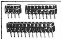
The TS strips provide positive screw activated clamping action, accommodate wire sizes 14-30 AWG (1.8-0.25mm). Pins are solder plated copper, .042 inch (1mm) diameter, on .200 inch (5mm) centers.
