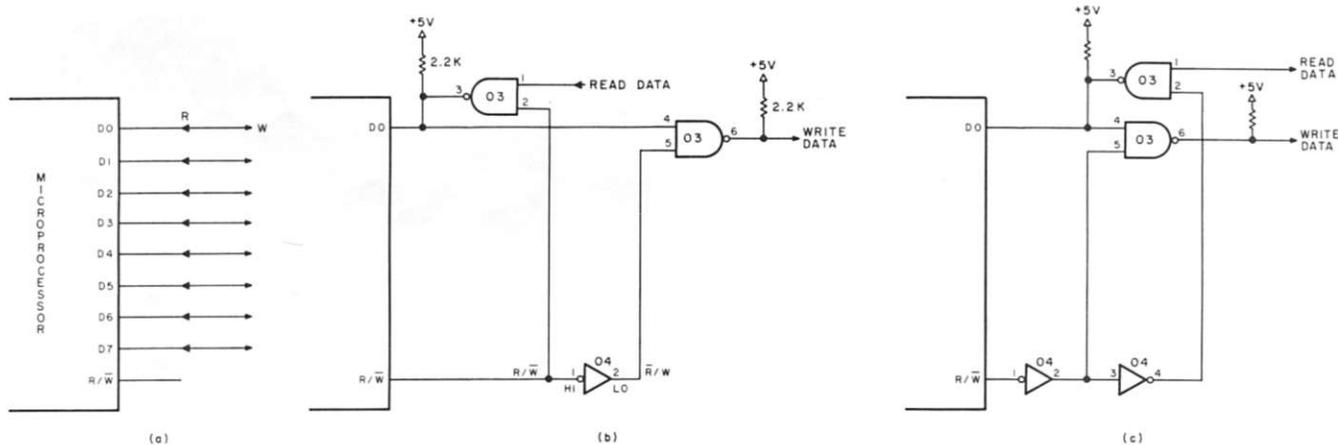
Fig. 7. Traffic control on the data bus.
