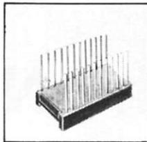
Dual-in-line package, 3 level wire-wrapping, phosphor bronze contact, gold plated pins .025 (0.63mm) sq., .100 (2.54mm) center spacing.
