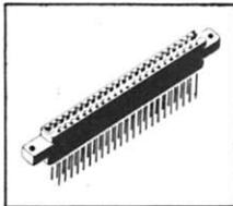
44 Pin, dual read out, .156" (3.96 mm) Contact Spacing, .025" (0.63 mm) square wire-wrapping pins.
