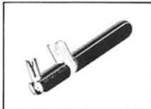
Easy to operate... place wires (up to 4) in stripping slot with ends extending beyond cutter blades... press tool and pull... wire is cut and stripped to proper "wire wrapping" length. The hardened steel cutting blades and sturdy construction of the tool insure long life.
