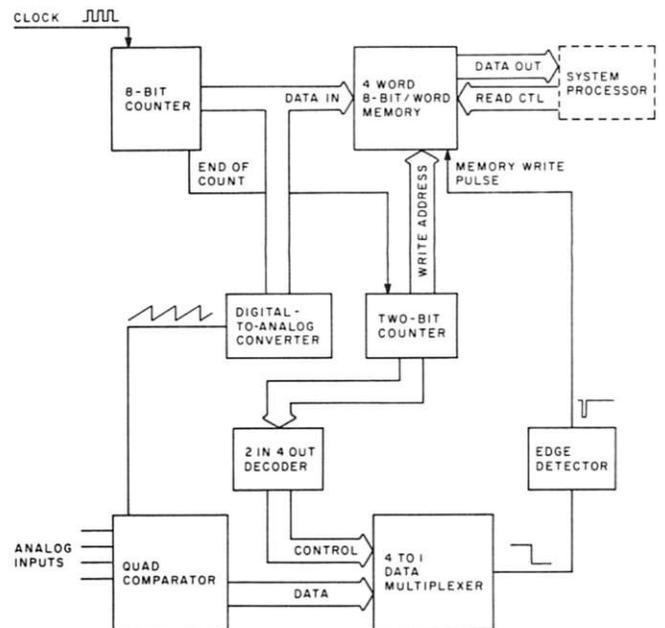
Fig. 1. Block diagram of the A/D converter.
