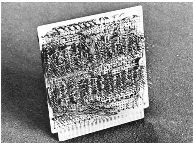
Photo 2. Circuits are wire-wrapped on a 44-pin board.
