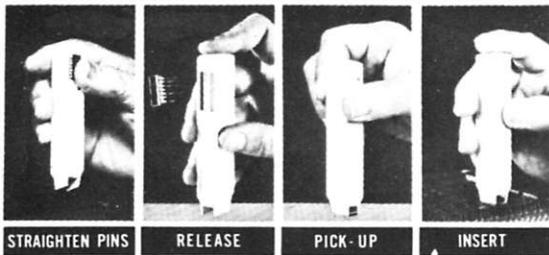
14-16 Pin Dip IC Inserter INS-1416 \$3.49
