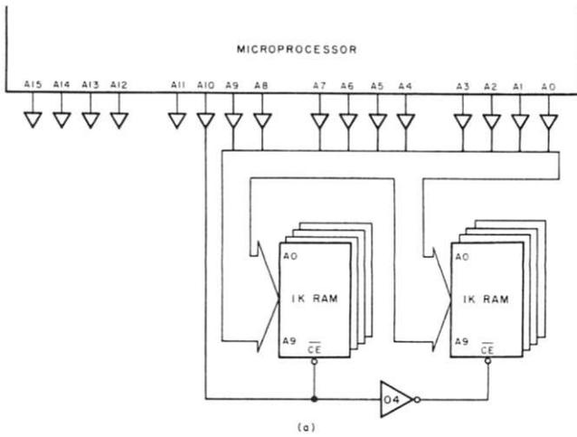
Fig. 2. Adding the second 1K RAM block.
