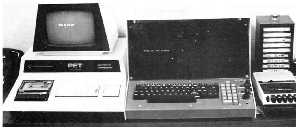
Photo 3. Now-defunct Sphere, right, is very similar to PET, left. Note the combined keyboard, TV, CPU, integral dual cassette controls and number pad. PET's cassette is built in.
