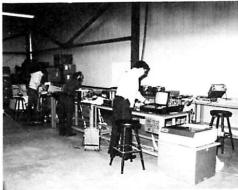
The CRT and CPU units are tested here as they are completed.
