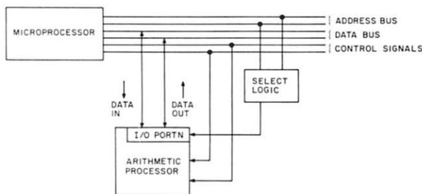
Fig. 1. An arithmetic processor in a microcomputer system.
